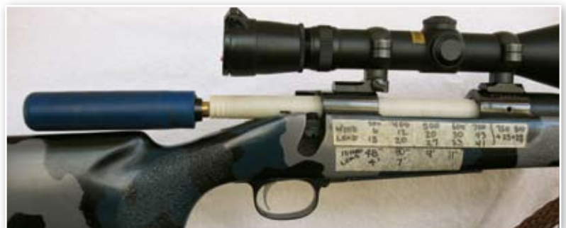
A cleaning-rod guide is a must-have item. It centers the cleaning rod with the bore and prevents damage to the chamber, throat and bore and prevents solvent from running into the chamber or trigger mechanism.
