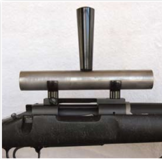
"Lapping" your scope rings smooths down the high spots of the bottom rings to closely align or center them with each other. Inexpensive lapping kits are available at gun supply outlets.
