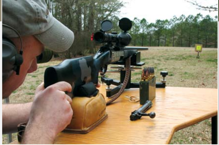
The authors always bore-sight newly scoped rifles, starting at 25 yards, by removing the bolt, centering the target through the bore, and checking to see that the crosshairs are also on the target.
